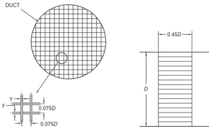
Fig. 2. Cell straightener geometry and dimensions [14]
