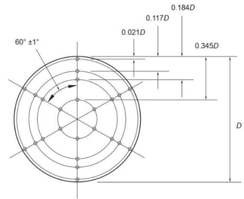
Fig. 3. Pitot tube traverse measurement points inserted into the test duct [14]
