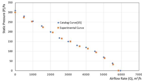
Fig. 5. Variation of static pressure with airflow rate of axial fan
