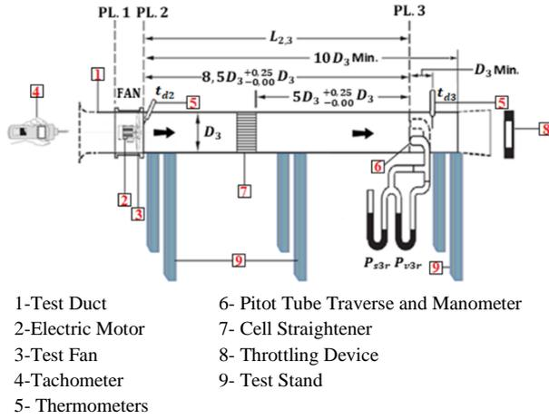
Fig. 1. Axial fan experimental set-up [14]
